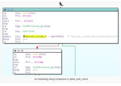
This is performing a stromp between the string pointer at offset 0xD0 inside the http\_request\_t structure and the string "xmlset\_roodkcableoj28840ybtide"; if the strings match, the check\_login function call is skipped and alpha\_auth\_check returns 1 (authentication OK).
