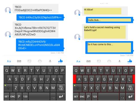
Fig. 2. An encrypted conversation displayed with BabelCrypt disabled on the left, and with BabelCrypt enabled on the right. Note that the background color of the keyboard and the overlay boxes change to indicate that a secure conversation is in progress.
